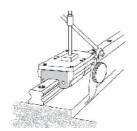
Fig 1.11.19 Use a Temporary Reference Surface
