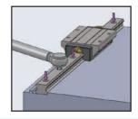
Fig 1.11.10 Full Tightening of Mounting Bolts
