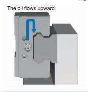
Fig 2.2.9 The oil sail against the gravity to lubricate the circulation path
