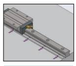
Fig 1.11.9 Tightening Set Screws
