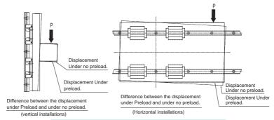
Fig 1.10.1 Relationship Between Preload and Displacement
