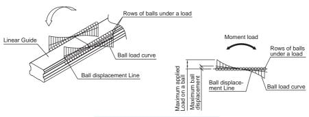
Fig 1.6.1 Ball Load Effected by a Moment
