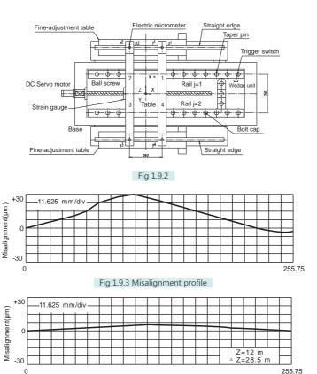
Fig 1.9.4 Horizontal displacement of the table
