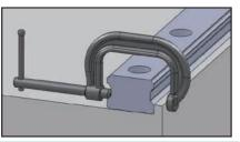
Fig 1.11.13 Mounting the master Linear Guide rail
