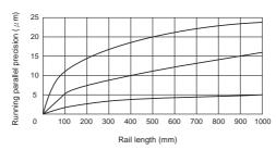
Fig 2.3.6 Running parallel precision slide relative to the rails datum
