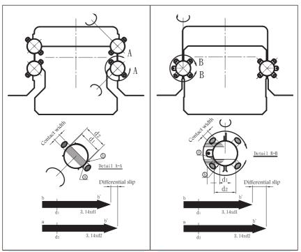
Fig 1.1.1 Four-Row Equal Load Ratting Design
