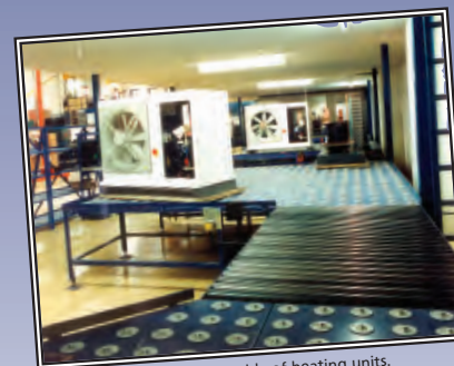
Ball units used for the assembly of heating units.
