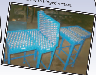
Ball table with hinged section.
