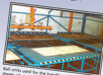
Ball units used for the assembly of heating units.
